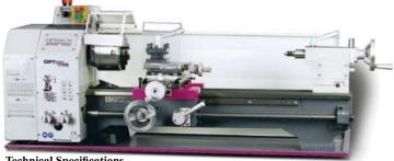
**Technical Specifications** 230 V / 1 Ph ~50 Hz Connection Driving motor spindle 750 W Spindle taper MT 4 Spindle hole Short taper Spindle seat Quadruple tool holder max. 13 mm Centre height 125 mm 550 mm Centre width Turning Ø over lathe bed 250 mm Bed width 135 mm 125 – 2,000 min-1 Spindle speed Number of steps 6 steps Travel top slide 70 mm Travel cross slide 110 mm
